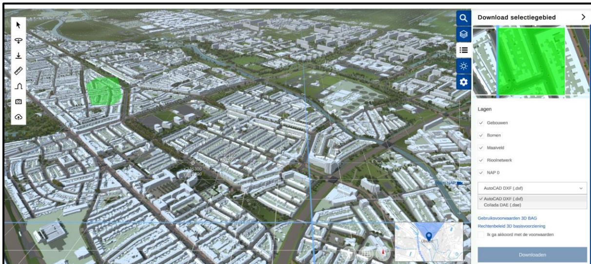
Figure 6: Users have the option to zoom download a desired area of the city in .dxf or .dae format
