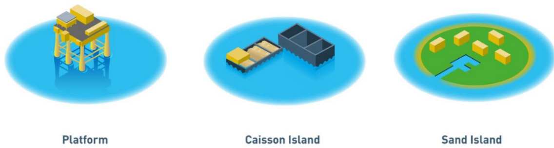
Figure 4: Possible foundation types for offshore energy hubs [48]
