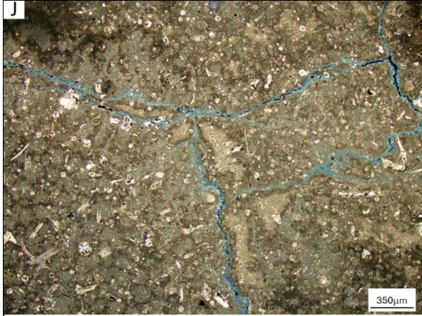
Figure 34: Plane-polarized light view (PPL) micrograph of TS_J from HRL_04 showing wackestone at 1055 m depth (HRL_04 well core). Open fractures are also observed in this thin section.
