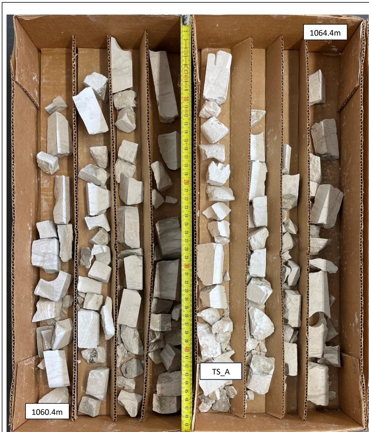
Figure 9: HRL-02 Core depth from 1060.4 to 1064.4. This represents the top of the core which is mostly chalky limestone with interbedded clay and minor sub-horizontal.
