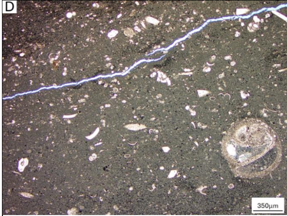
Figure 22: Plane-polarized light view (PPL) micrograph of TS_D from HRL_02 showing wackestone to mudstone at 1069.6m depth (HRL_02 well core). Open fractures are also observed in this thin section.
