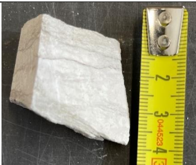
(A): Depth: 1062.15. Chalky limestone with sub-horizontal fractures interbedded by clay.
