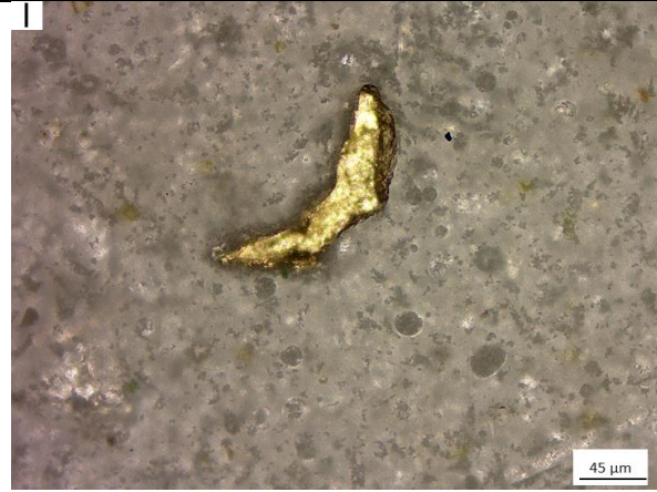
Figure 35: Plane-polarized light view (PPL) micrograph of TS_J from HRL_04 showing phosphatization in bioturbation.
