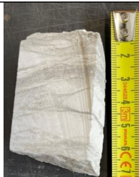
(B): Depth: 1062.3. Chalky limestone with low angle interbedded clay no fractures present.
