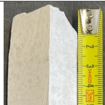
(B): Depth: 1065.95. Homogeneous chalky limestone no fractures and no clay interbedded.
