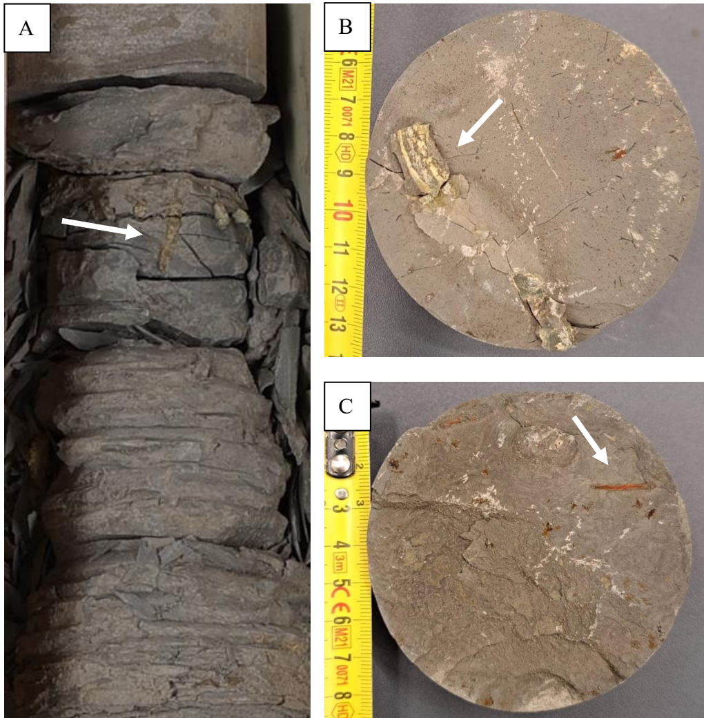
Fig. 12. Example of the fossil and bioturbation content of the Lower Jurassic in the Molenbeersel borehole. A) Example of a burrow (white arrow) in the lowermost interval of the core at 1718.84 mbs. The burrow presents pyritization in the interior part of the bioturbation. B) Example of a pyritized bioturbation (white arrow) at 1310.64 mbs. C) Example of oxidized organic matter (white arrow) at 1313.7 mbs.
