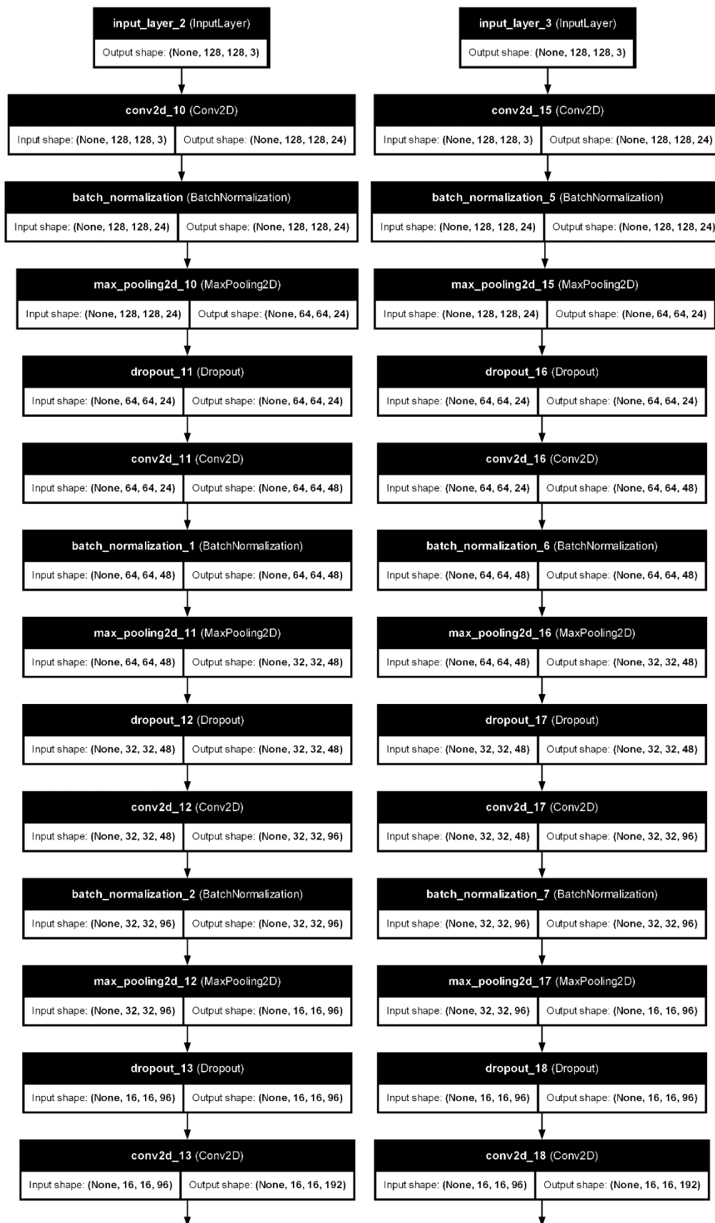
Figure B10: Upper half of the final (D)CNN architecture.
