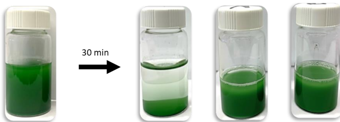
Figure 13 Pictures of \text{Cr}_2\text{O}_3 dispersions. picture on the left is a freshly dispersed sample. Three pictures on the right show samples after 30 minutes. Sample 1 only contains \text{Cr}_2\text{O}_3 (2wt%), sample 2 contains NaCas and \text{Cr}_2\text{O}_3 (1 wt%, 2 wt%) and sample 3 contains whey proteins and \text{Cr}_2\text{O}_3 (1 wt%, 2 wt%)
