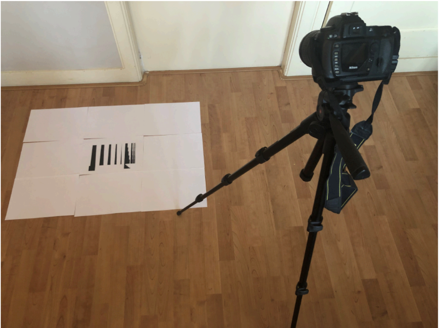
Figure 2.9: An impression of the setup used to photograph the chromatometer through the historical prisms held in Museum Boerhaave, Teylers Museum, and the University Museum Utrecht. The chromatometer is placed on the floor between sheets of white paper to prevent influence of the colour of the floor. The photos were made with a Nikon D70s camera on a tripod, 1,5 meter above the chromatometer on the floor. All prisms were held at a distance of 2-12 cm from the camera lens, with one face of the prism aligned with the floor, and the apex angle of the prism perpendicular to the orientation of the camera. (Photo by Dr. Hieke Huistra.)
