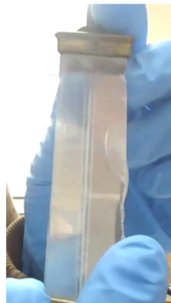
Figure 2.13: Two half circles of striae visible in prism Li-77. (Photo above by the RCE; photo to the right by Dr. Hieke Huistra and the author.)
