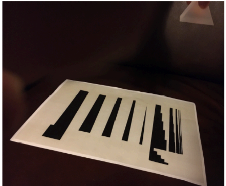
Figure 2.18: Coloured bands visible through my flint glass prism when moved closer to the chromatometer (left). Position of the flint glass prism above the chromatometer to perceive these bands (above). (Photos by the author.)
