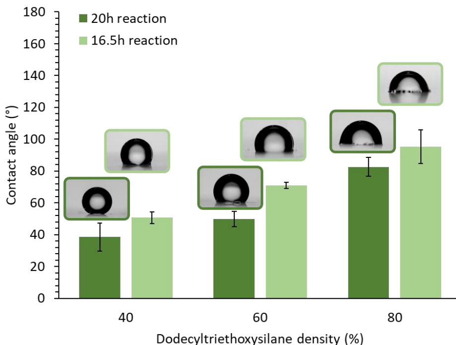
Figure 46 Contact angles for the DTES functionalized particles using a slightly different reaction time.
