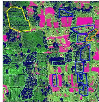
(b) The same sub-area with vegetation mask (pink) and shadow mask (dark blue) applied. Pink areas designate non-vegetated parts.
