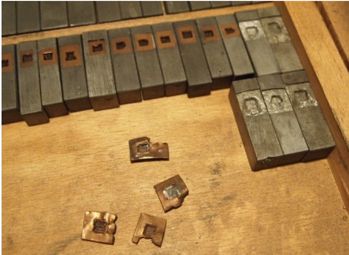
Figure 11 Copper layer on electrotyped matrix. These electrotyped copper matrix-eyes came loose from their “bodies”, presumably a zinc alloy. Copper does not bind well with zinc and has to be tinned at the backside. Object: matrices from Gerstenberg type foundry in Germany. Photo: Indra Kupferschmid, 2015. Source: https://www.alphabetes.org/making-matrices/ (accessed on 1 May 2021)
