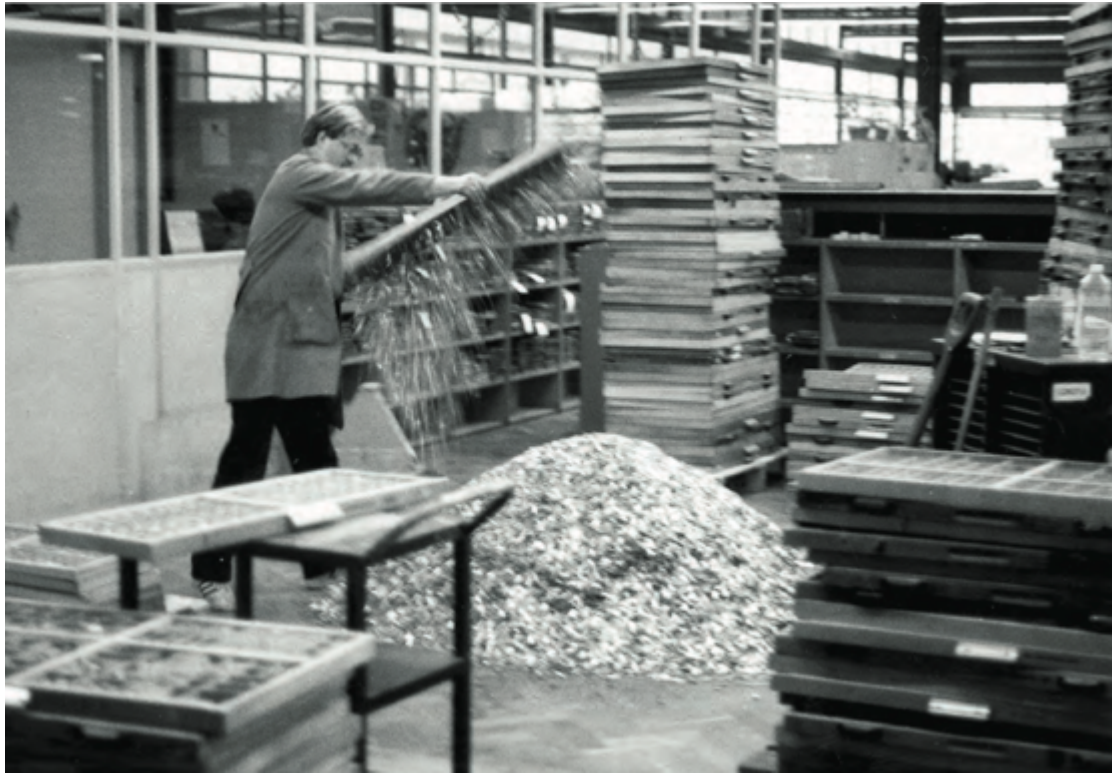
Figure 33 The end of the type-metal era in the eighties: a typesetter empties the type cases. Manual typesetting, only for works in Chinese and Japanese, continued at Brill until 1987. Brill archives in UvA special collection.
