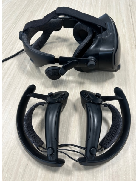
Figure 2 A photo of the Steam Valve Index VR HMD and the controllers, left and right.
