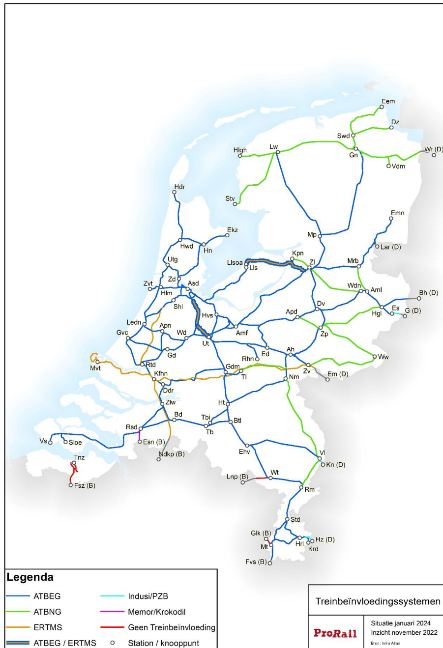
Figure 6.1: Distribution of various NTC systems across the Dutch railway network (ProRail, 2023, p. 217). The dual signalling track between Amsterdam (Asd) and Utrecht (Ut) is indicated in blue and orange. Other railway tracks, including the track between Lelystad (Lls) and Zwolle (Zl), are out of the scope of this thesis.
