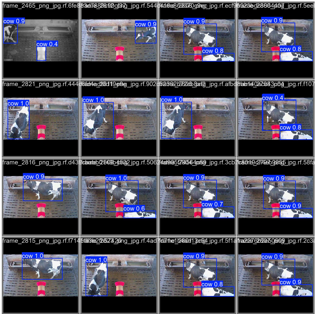
Figure 5.2: Test batch predicted bounding boxes for several frames. The confidence level is given for each bounding box. This indicates the level of confidence of the cow class.
