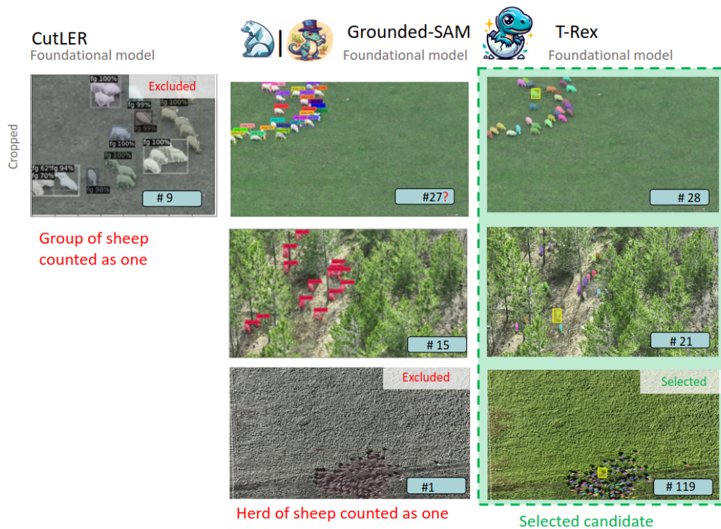
Figure 3.2: The counting performance of the tree foundational models varies depending on the complexity of the scenario. T-Rex performance is remarkable even in complex scenarios with numerous clustered sheep. Other models such as CutLER, Grounded-SAM or Grounding-DINO, were only able to count multiple objects in more simple scenarios.
