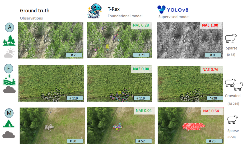
Figure 3.8: The figure shows the counting performance of some selected cases for a qualitative analysis. Row A displays a forest scenario under overcast weather where only T-Rex is able to count sheep blended with the background. Following the same trend, T-Rex made a perfect prediction (NAE 0) while YOLOv8 had a poor performance with NAE 0.76. Lastly, although pen scenarios such as row M pose a challenge, given the bigger size of the sheep, T-Rex almost scored the highest prediction.
