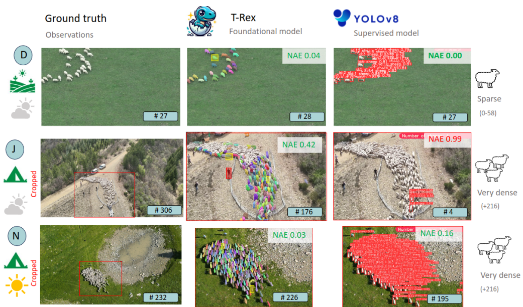
Figure 3.9: This figure highlights the role of the complexity of the scenario. T-Rex and YOLOv8 counted the herd successfully when only 27 sheep, relatively scattered, appeared on a clear pasture. However, as the number of sheep increased, it was required to crop the image to run both models.
