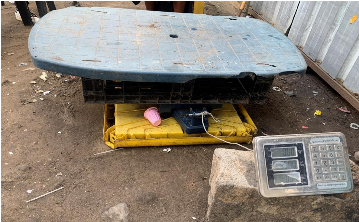
Figure 19 shows an example of scale aspired by aggregators, it has been modified with an old table to widen the surface area.
