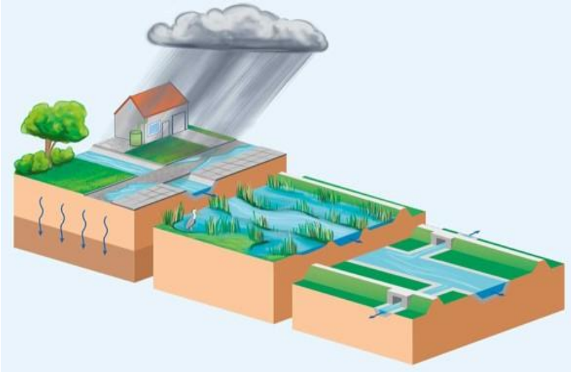
Figure 2.3: Three-stage strategy of water retention, storage and discharge in order
