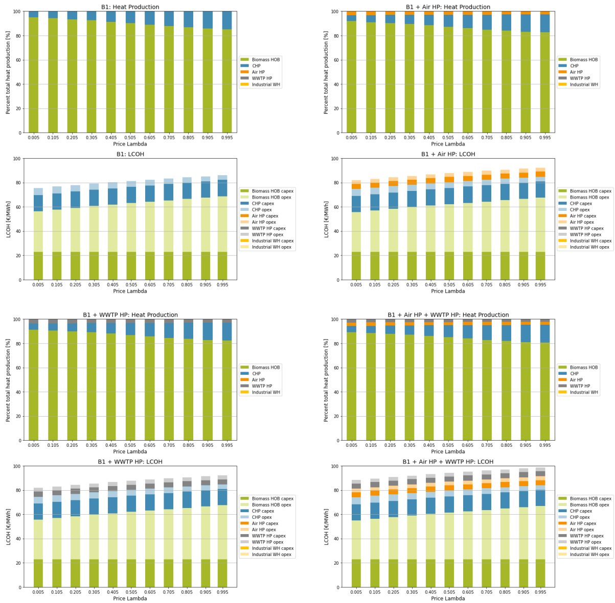
Figure B.1 Heat output per technology and levelized cost of heat (LCOH) broken down into capital expenditure (CAPEX) and operation expenditure (OPEX) across energy scenarios for system configurations in scenario B1.
