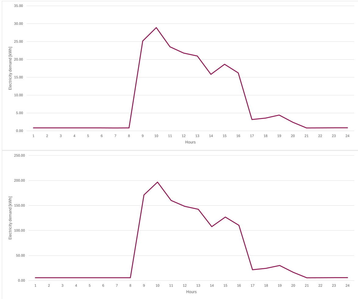
Figure 14. Electricity demand distribution in kWh over 1 day (11-1-2022). The top graph is the Luc Stevenschool and bottom graph is De Weide Vleuten.
