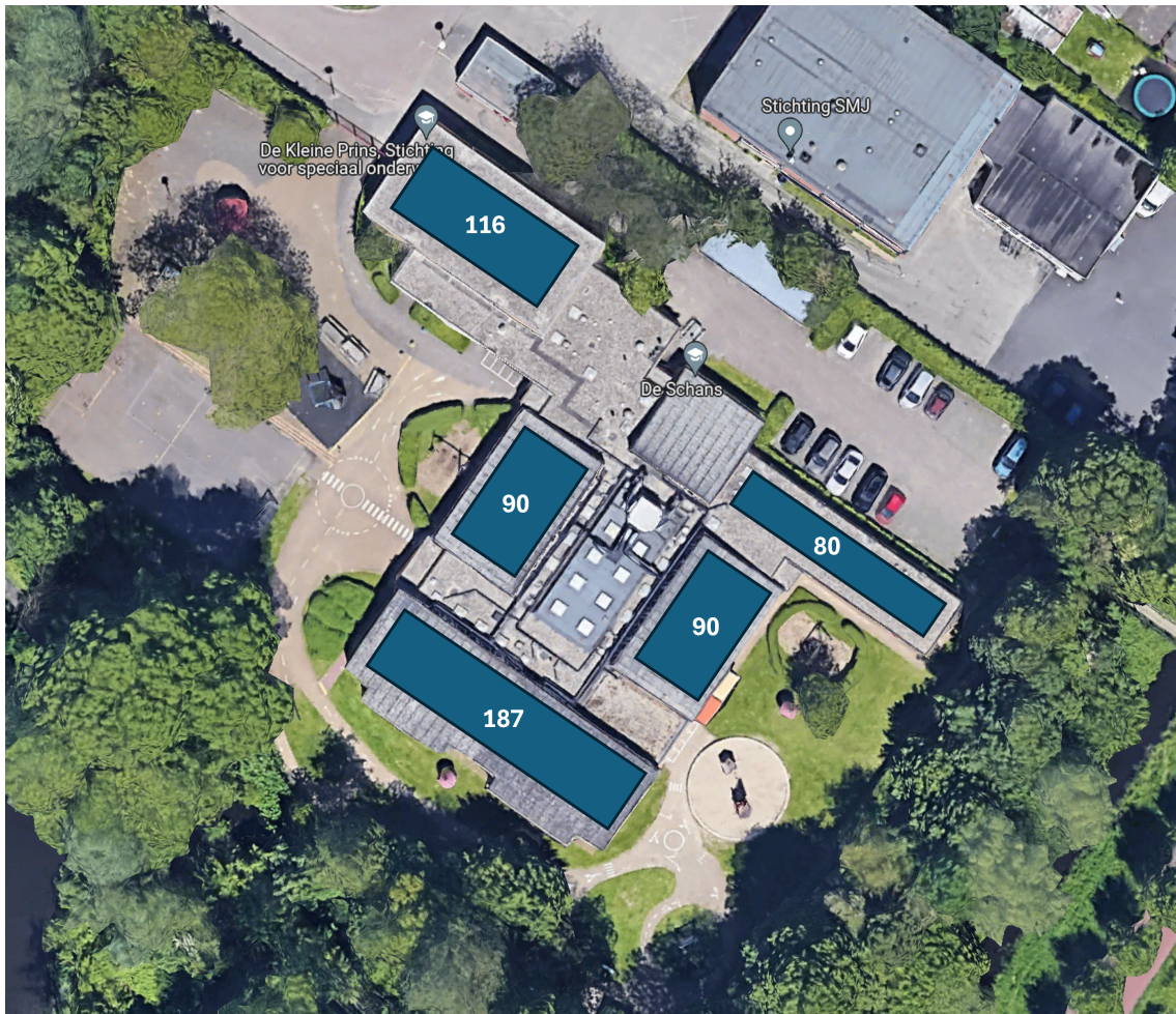
Figure K1. Top view of primary school De Kleine Prins, with available space for solar panels, obtained from Google Map.
