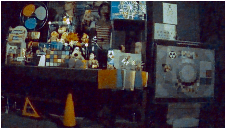
Figure C.16: R04: Restormer model without progressive learning, with the loss based on SCUNet loss, with Conv transpose upsampling. Result on 63dB noise real sensor data.
