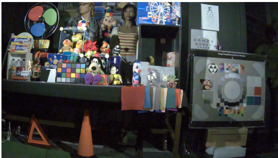
Figure C.8: R02: Restormer model with the loss based on SCUNet loss, with Conv transpose upsampling, progressive learning. Result on 45dB noise real sensor data.
