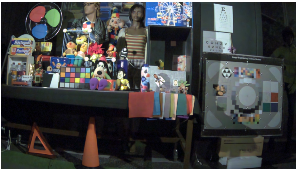
Figure C.2: R02: Restormer model with the loss based on SCUNet loss, with Conv transpose upsampling, progressive learning. Result on 32dB noise real sensor data.
