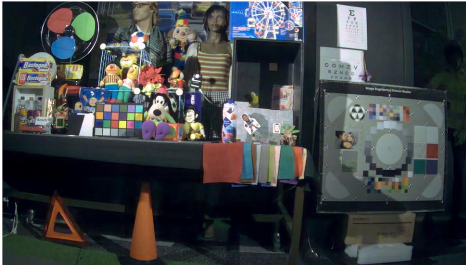
Figure E.7: KD07: Compressed SCUNet model using 2 blocks for each resolution step, with feature-based and response-based knowledge distillation ( w=10 ) from S05. Result on 32dB noise real sensor data.
