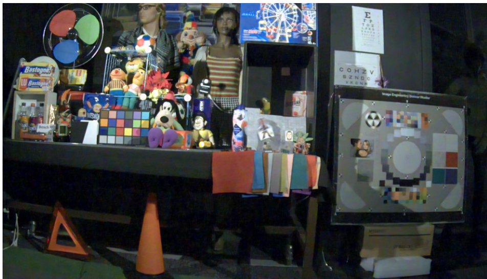
Figure C.9: R03: Restormer model with the overall skip connection, the loss based on SCUNet loss, Conv transpose upsampling, progressive learning. Result on 45dB noise real sensor data.
