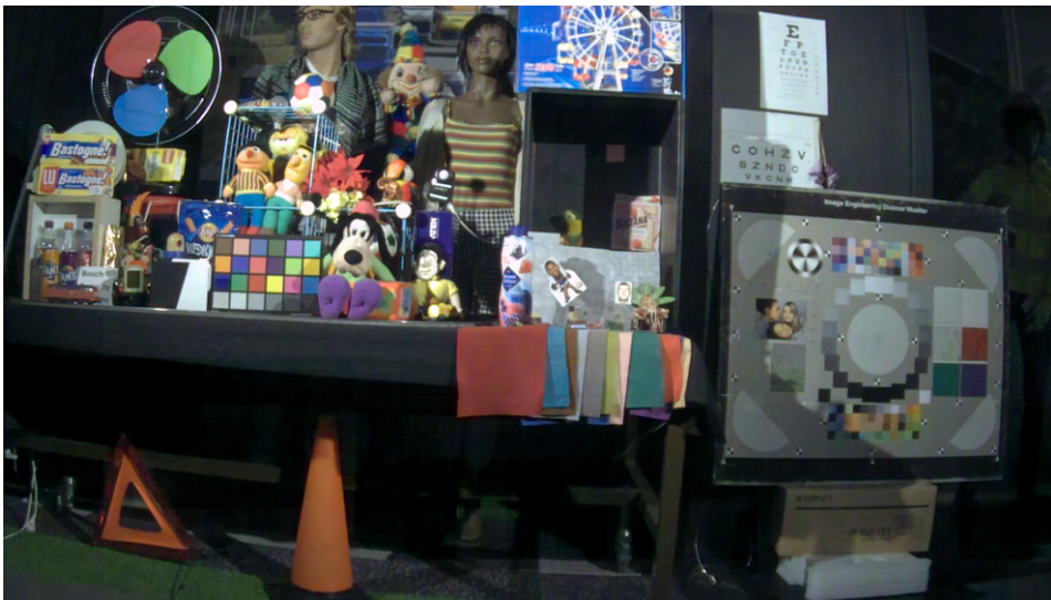
Figure E.6: KD06: Compressed SCUNet model using 2 blocks for each resolution step, with feature-based knowledge distillation ( w=1 ) from S05. Result on 32dB noise real sensor data.
