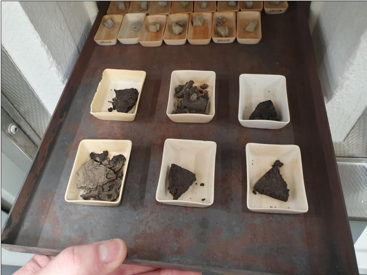
Figure 16 shows the darker core samples that have been dried and need to be ashed for LOI. The smaller crucibles contain ashed samples which are significantly inferior in mass and size (L. Bonanno, 2023).
