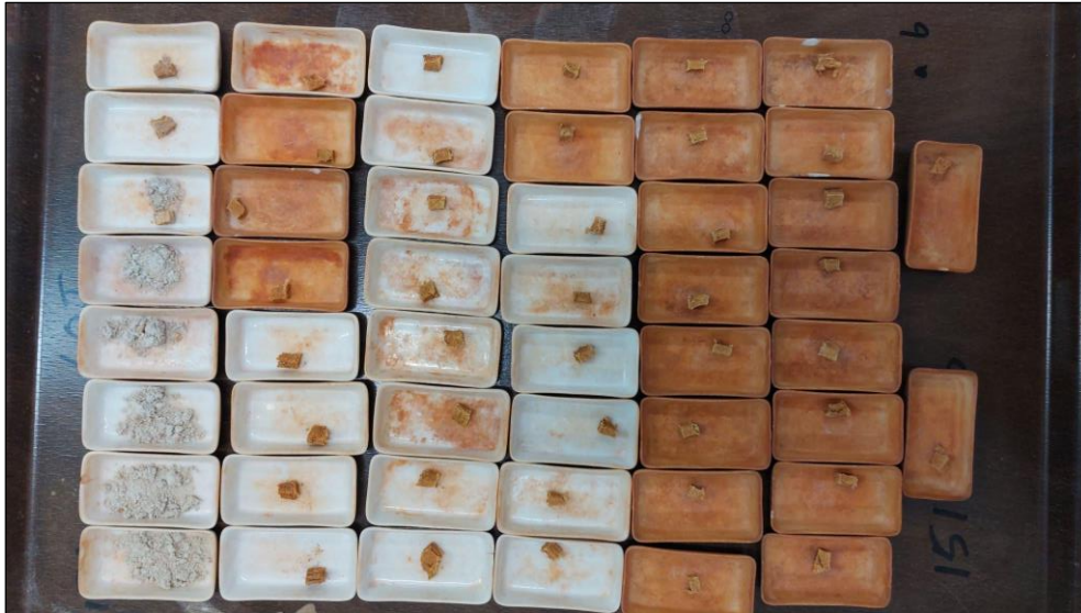
Figure 17. A tray of ashed samples in small crucibles are ready to be weight measured and fractionated with the sequence of sieve filters (L. Bonanno).
