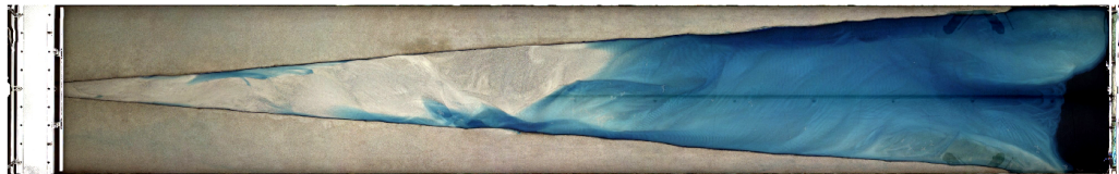
Figure 8.2: Calibration Orthomosaic depth at weir height 75.70mm
