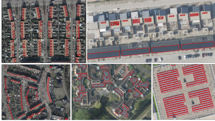
Figure 1.1: Example output of a PV segmentation algorithm, taken from [5].
