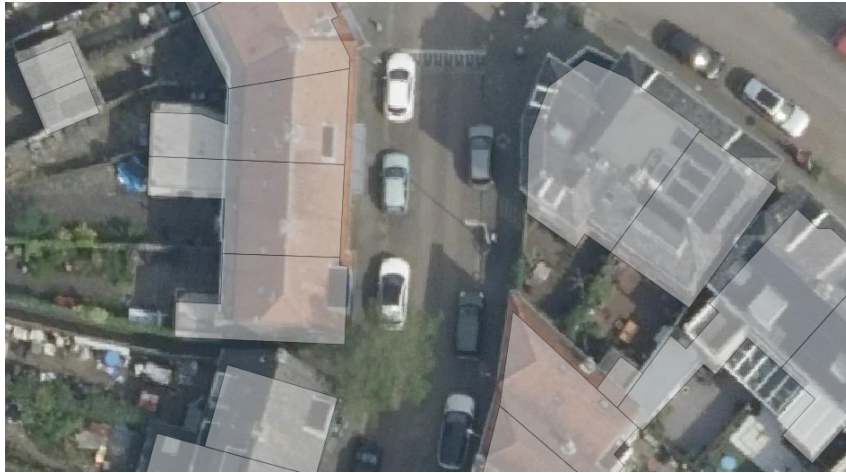
Figure 4.3: Misalignment between BAG polygons and aerial image. BAG polygon in grey.
