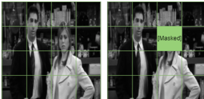
Figure 3.3: Example of the process of masking tokens for the spatial dimension of the video modality. Each video is divided into a 4 x 4 grid. For each frame in the video, the patches at the same location get masked.
