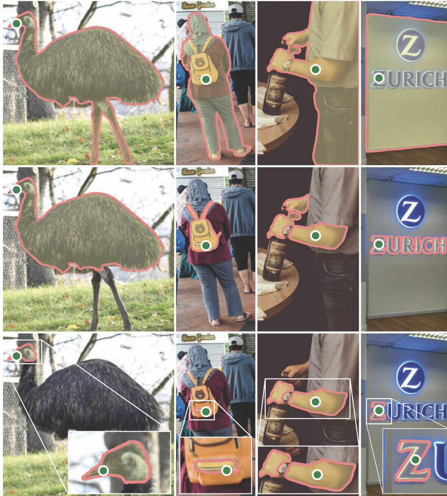
Figure 6: Each column shows 3 valid masks generated by SAM from a single ambiguous point prompt (green circle). (Directly from SAM paper [33])
