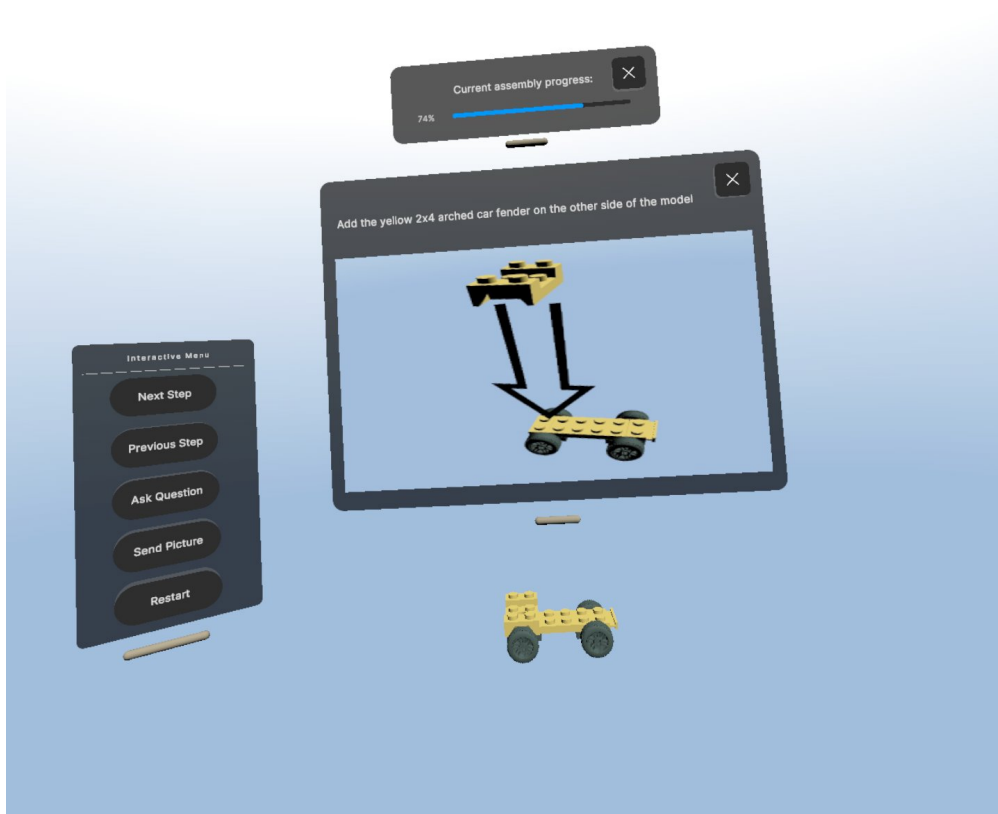
Figure 10. User view after pressing the 'Send Picture' button. The dialogue agent sends a picture from the manual as well as textual assembly instructions.
