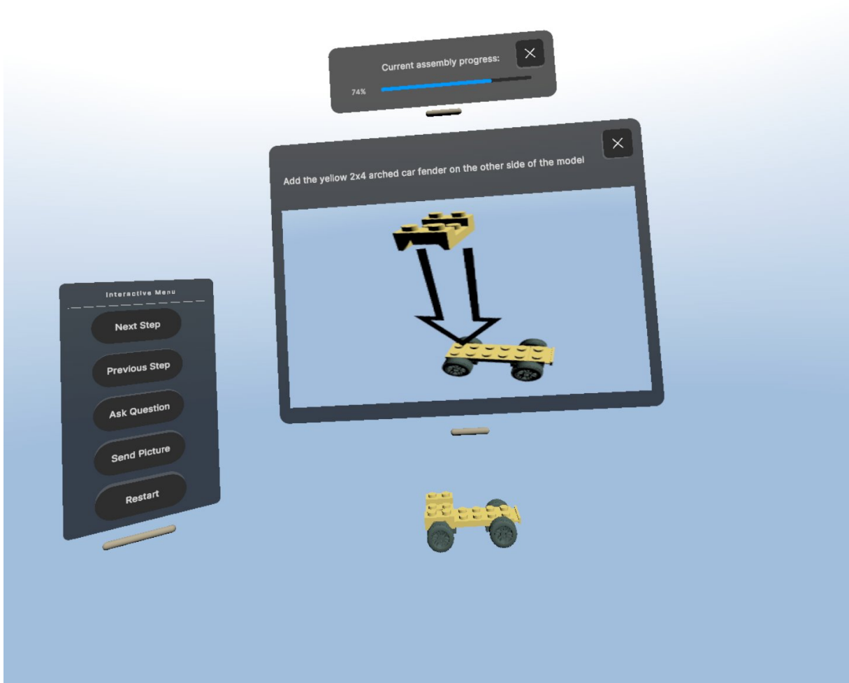
Figure 18. User view after pressing the 'Send Picture' button. The dialogue agent sends a picture from the manual as well as textual assembly instructions.
