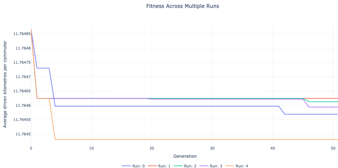
Figure 5. Generational fitness over multiple runs of the P&R parking fee optimisation model based on the best performing hyperparameter values.
