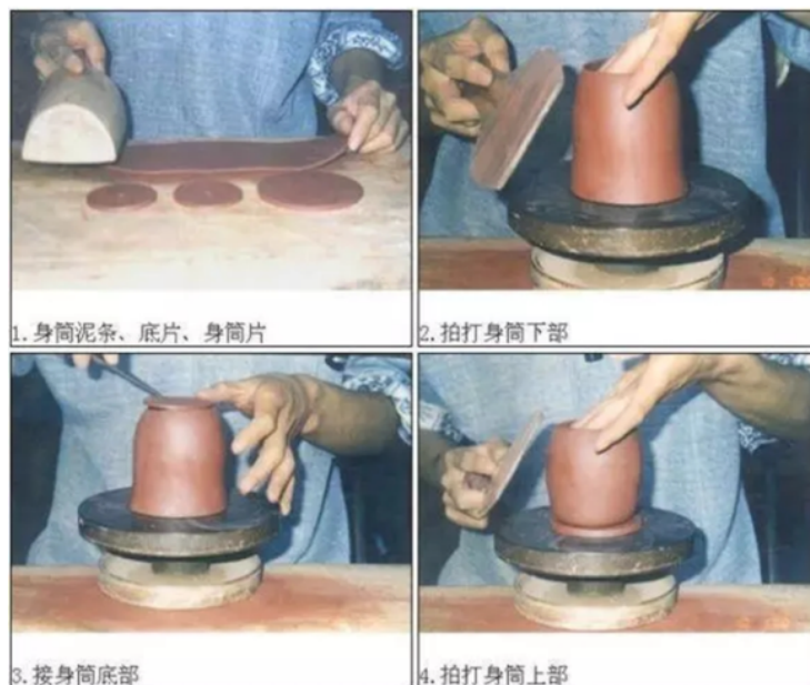
Fig. 2 Diagram showing the general production processes of Da Shentong technique in Yixing. Photos retrieved from “ban shougong he quan shougong de qubie he gongyi tezheng” (The differences between the semi-hand-made teapots and hand-made teapots), Yihu Website, accessed 5 Oct. 2023, https://www.sohu.com/a/123973496_213539 .
