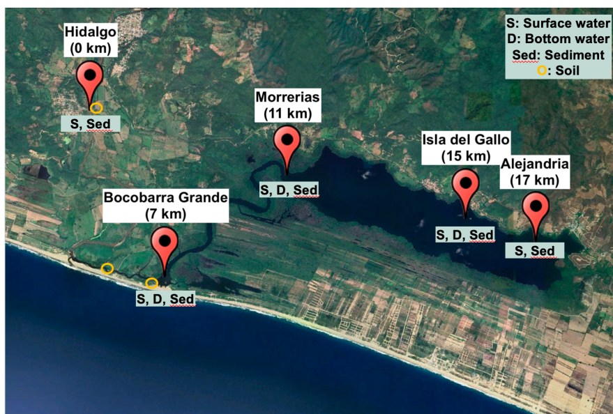
Figure 5: Location of the Manialtepec Lagoon with the position of the five sampling sites (red arrows). Hidalgo is seen as the starting location (0 km) in the Manialtepec river and the four other locations have distances relative to Hidalgo indicated. For each site it is indicated what type of samples were taken there: surface water (Sur), bottom water (D), sediment (Sed), and soil (yellow circle).
