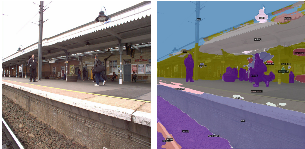
Figure 13: View of camera 3 of part of the station with Detectron2 inference.
