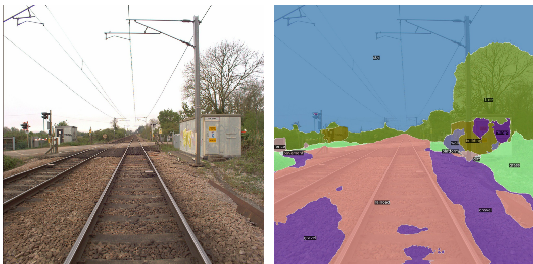
Figure 14: Camera image and inference of part of the track with a big electrical box.
