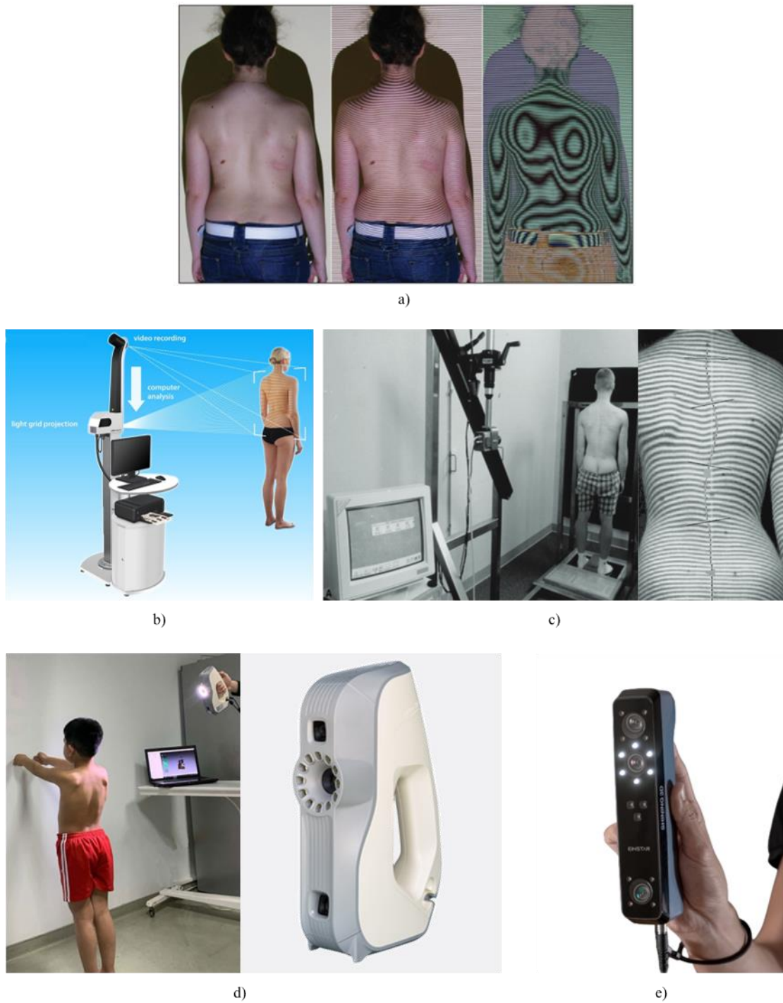
Fig A1. Examples of some common surface topography systems for the evaluation of scoliosis. a) Moiré method (back image, projection of parallel lines, Moiré image reconstruction) [21]. b) Formetric 4D system (Diers International GmbH, Germany) [22]. c) Quantec Shape Imaging System (Quantec Image Processing, United Kingdom) [7]. d) Hand-held 3D scanner Artec EVA (Artec Group 2013, Luxembourg) [8], [23]. e) Hand-held 3D scanner Einstar (Shining 3D, China) [15], employed in this research study.
