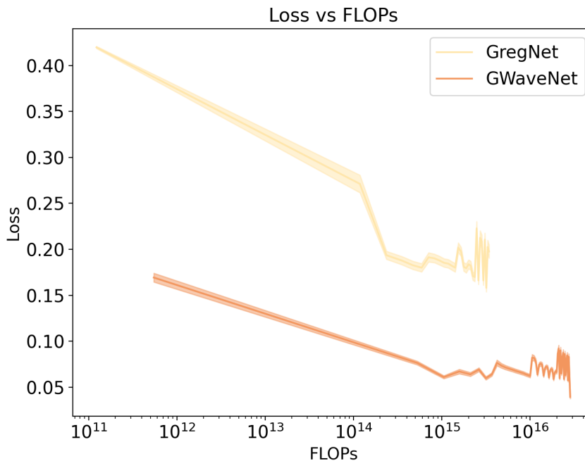
Figure 4.3: Training losses over number of FLOPs for GregNet (cream) and GWaveNet (orange). We present the average loss per epoch for the cumulative amount of FLOPs and the corresponding 3\sigma error. The vertical axis is in logarithmic scale.
