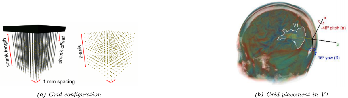
Figure 8. Illustration of electrode grid configuration (8a) and placement (8b) van Hoof et al. (2024, p. 4).
