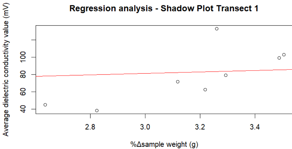
Figure 35. Regression analysis on obtained dielectric conductivity and %Δsample weight values Shadow plot primary transect 1.
