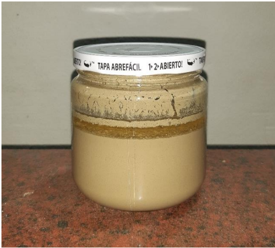
Figure S3. Jar with soil sample, water, and detergent, 24 hours after mixing. Flash used.
