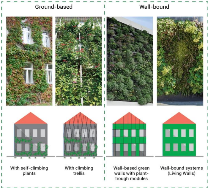
Figure 1. Ground-Based Green Facades (GFs) and Wall Bound Living Wall Systems (LWS). Adapted from the European federation of Green Roofs & Walls.
