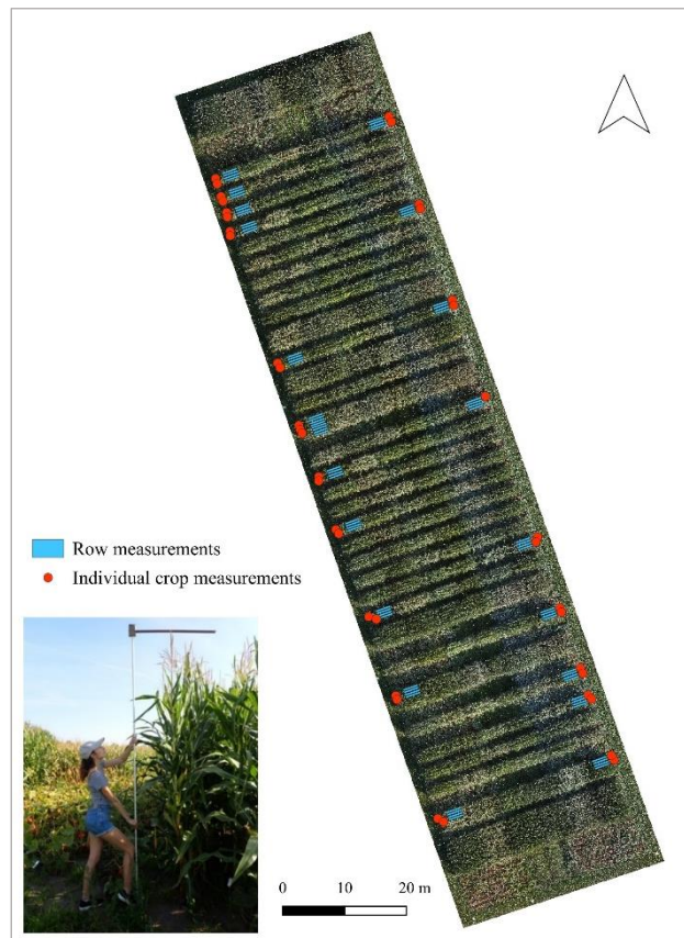
Figure 8: Method and location for maize height measurement: from base to tassel top.
