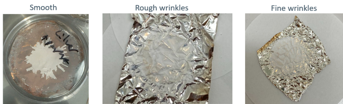
Figure A.3: PMMA on smooth, roughly wrinkled, and finely wrinkled Ag foil
