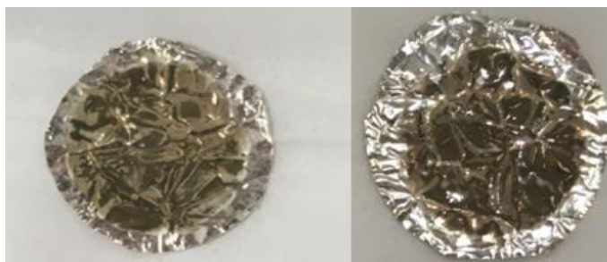
Figure A.24: Pictures of 2 porous Ag catalysts. The dark regions are porous, and the light regions are non-porous
