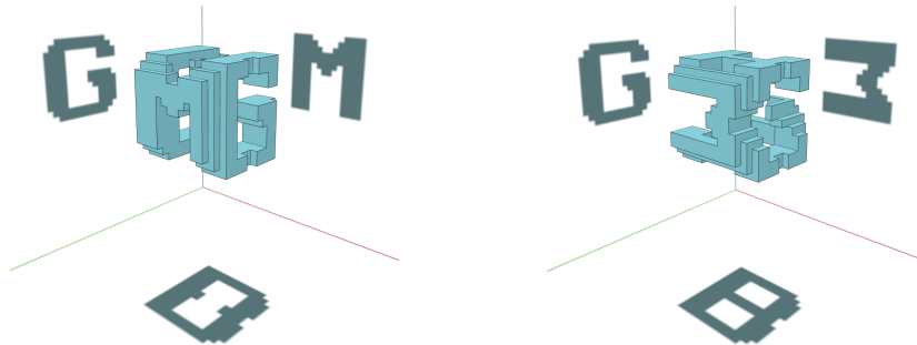
Figure 5: An example where rotating a shape plane results in more accurate shadows. When the M is rotated 90^\circ degrees clockwise, the shadow of the B becomes whole, unlike when the M is not rotated.
