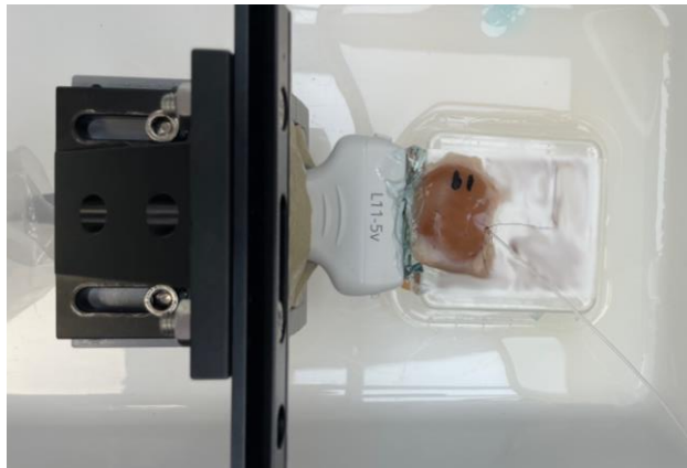
Fig 8: Rabbit kidney during ultrasound acquisition: The main artery is connected to a hose through which the microbubble suspension was pumped. The Transducer is mounted to the same platform as in Supplementary figure 4.
