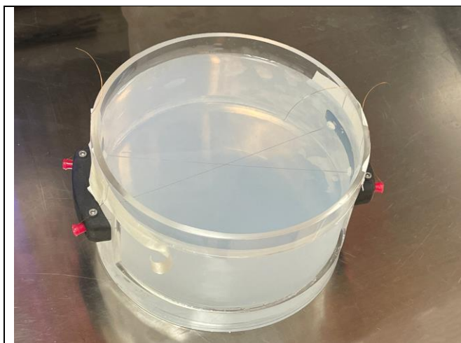
Fig 1: Photo of phantom during its creation. To create the wall-less tubes, copper wires were spanned across the phantom. After the PAA solidified the wires were pulled out and left tubes in the PAA.
