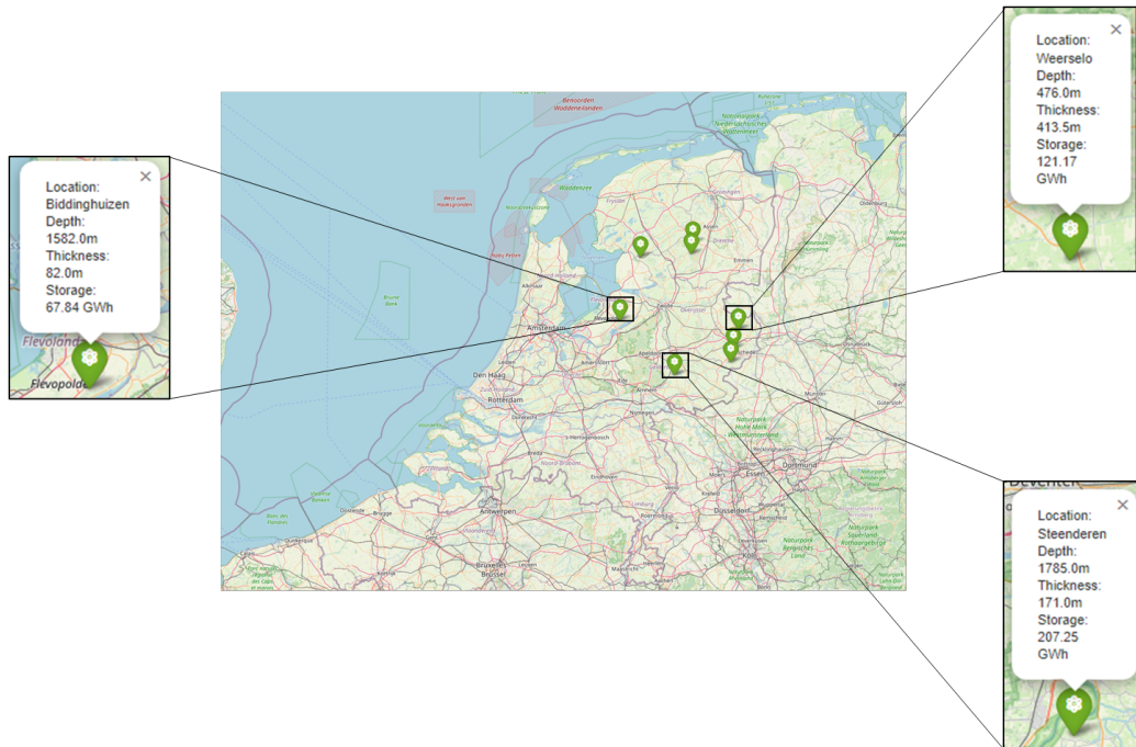
Figure 15. An overview of the map generated within the model. Each of the green pins represents a borehole which is used for input data. The image also shows certain data which is included on the map for each location.
