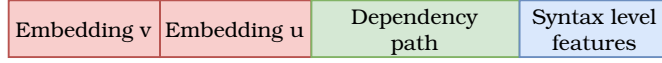
Figure 9: An overview of the feature vector representation of action (v, u) . It is a concatenation of word embeddings of the 2 terms, the dependency path of these terms based on the background corpus, and their syntax level features into a single vector.
