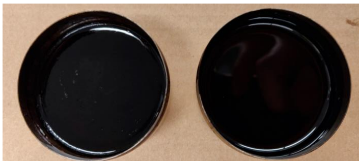
Figure 4 Visual comparison of prototype circular and bio-based asphalt binder (left) and conventional bitumen (right) (Hendrikse et al., 2023).
