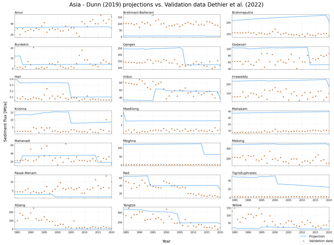
Figure 4.2: Absolute magnitudes of Dunn et al. (2019) projections and of the validation data of Dethier et al. (2022) for rivers in Asia
