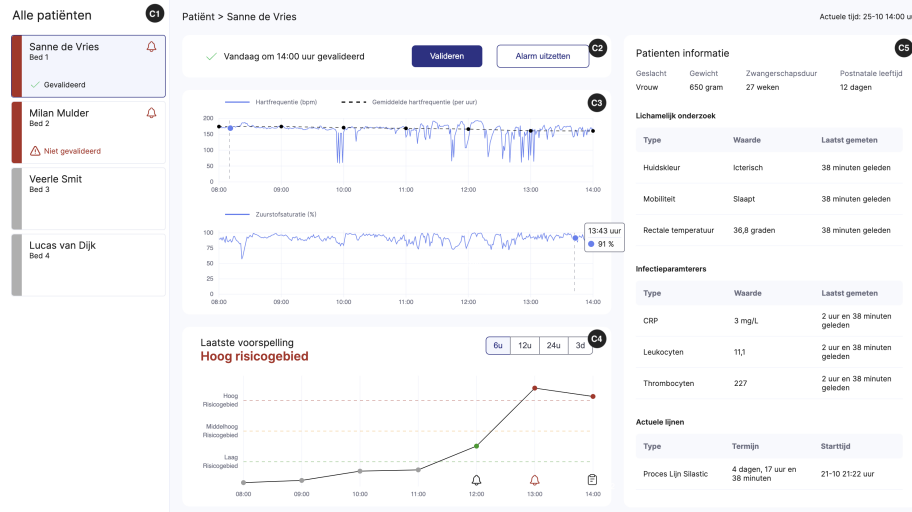
Figure 21: Dashboard design of the high-fidelity web application prototype. The dashboard contains an overview of the patients (C1), alarm notification (C2), vital signs (C3), prediction trend (C4) and a summary of the patient information (C5). Note: patient names & dates are not real.
