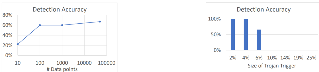
Figure 2.9: Detection accuracy of Neural Cleanse based on the number of data points used and the size of the trojan trigger [20]
