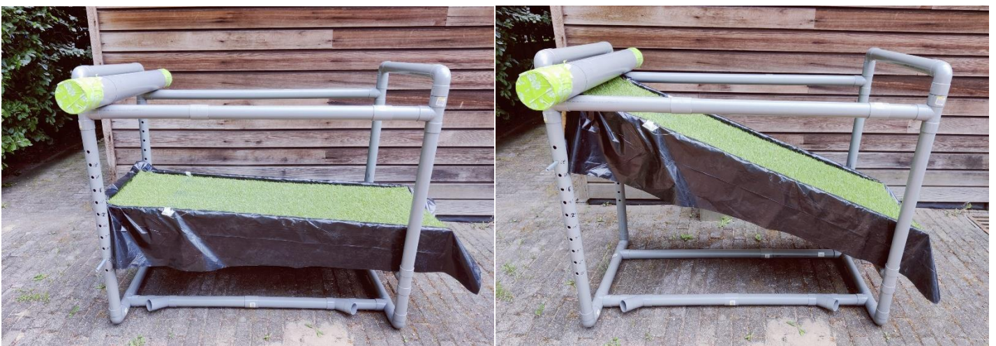
Figure 3 Experimental setup used for this experiment. A 0.16 m foam board layer was used with a plastic cover on top of it to prevent water seepage on the sides. A layer of synthetic grass was used to mimic grass. For the inflow of water, a perforated tube was built and placed on top of the frame. Furthermore, different slopes were created such that different scenarios can be obtained. The left figure shows the setup at the lowest angle (2°) and the right figure at the highest angle (20°).
