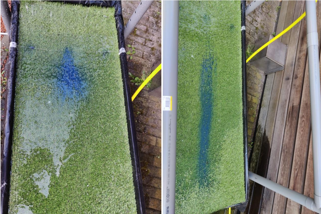
Figure 6 A dye tracer test was applied to measure the water velocity. First, a specific location was chosen for the placement of the dye. This was marked with a white string taped on the sides as shown in the figure. Then a dye was placed on the specified location. After that, the tip of the dye cloud was measured until it reached the end of the experiment. This process was repeated three times. The dye was first poured on the left side, then in the middle and lastly on the right side.
