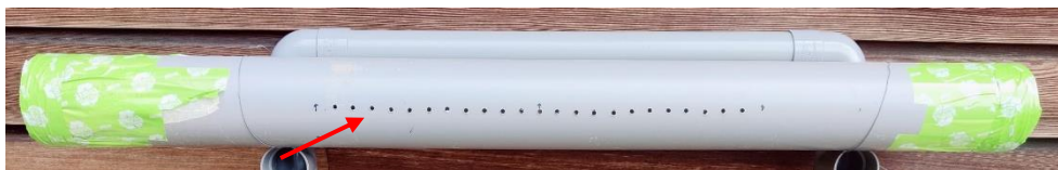
Figure 5 A perforated PVC tube was used for the equal distribution of water. 2 mm holes were drilled along the length of the PVC tube. Water will flow into the tube and spread along the holes created.
