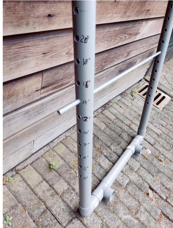
Figure 4 Holes were drilled on both sides of the setup based on the angles used. The angles ranged from 2 - 20°. For a better visual representation, the angles were written on the sides. A rod was used to adjust the specified angle of a test.
