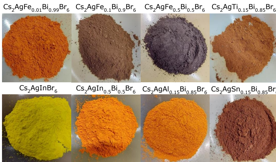
Figure 33. Images of a selection of the composite DPs that are synthesized with the ball mill. The differences in color demonstrate the effect of atomic exchange on the optical properties.
