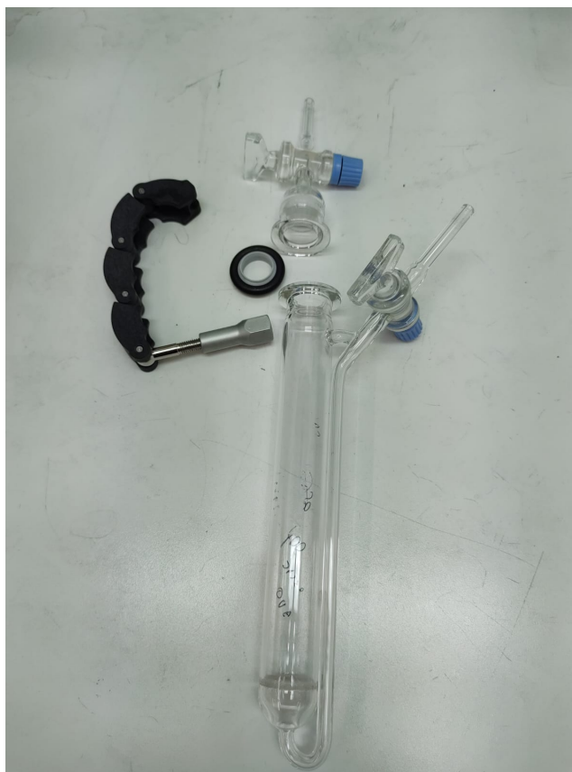
Figure A.6: Reactor used for calcination and reduction experiments
