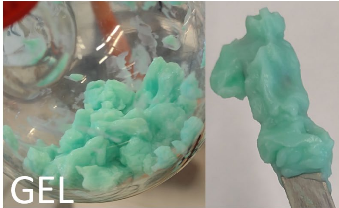
Figure 47: Appearance of synthesis product after washing & centrifugation. Left: clay appearance at low NaOH wt% (5-7). Right: gel appearance at high NaOH wt% (10)
