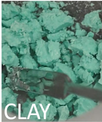
Figure 47: Appearance of synthesis product after washing & centrifugation. Left: clay appearance at low NaOH wt% (5-7). Right: gel appearance at high NaOH wt% (10)
