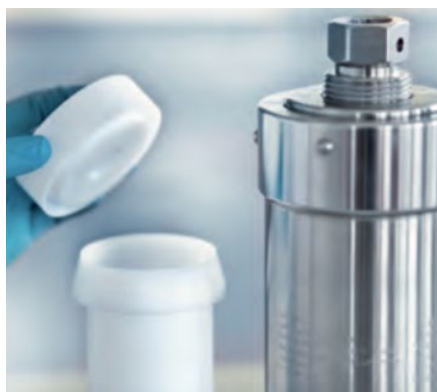
Figure 12: Picture of the DAB-3 autoclave and teflon liner used for hydrothermal synthesis of Ni phyllosilicate nanotubes. 56 Maximum pressure: 300 bar. Maximum temperature: 250 °C.
