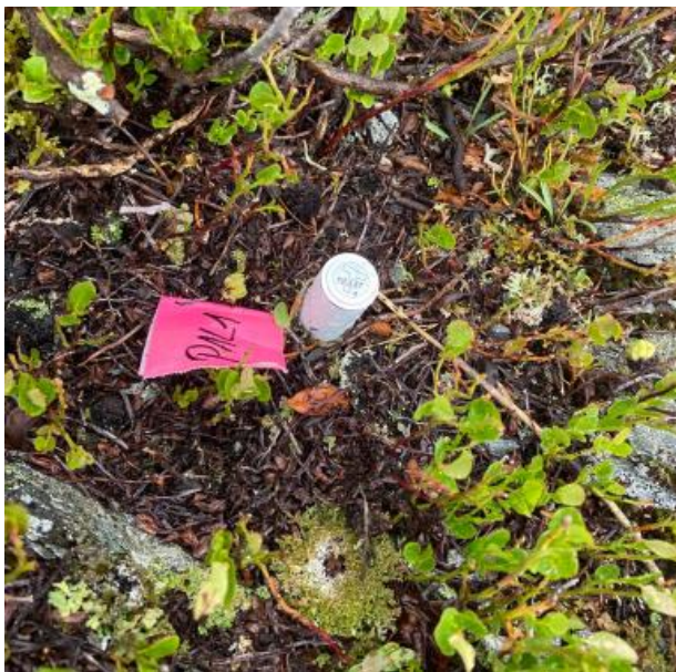
Figure 10: TMS-sensor, placed as surface sensor inside a plot (picture by Dick van de Lisdonk).
