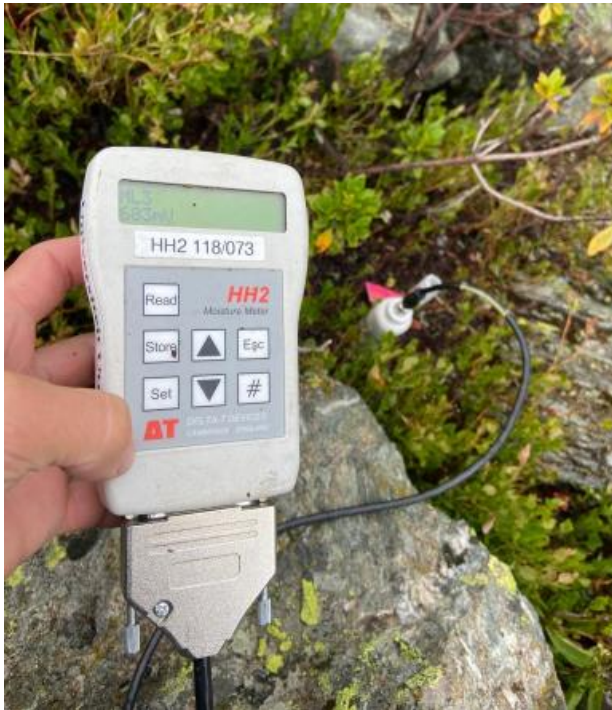
Figure 11: Theta-probe measurement executed inside a plot (picture by Dick van de Lisdonk).
