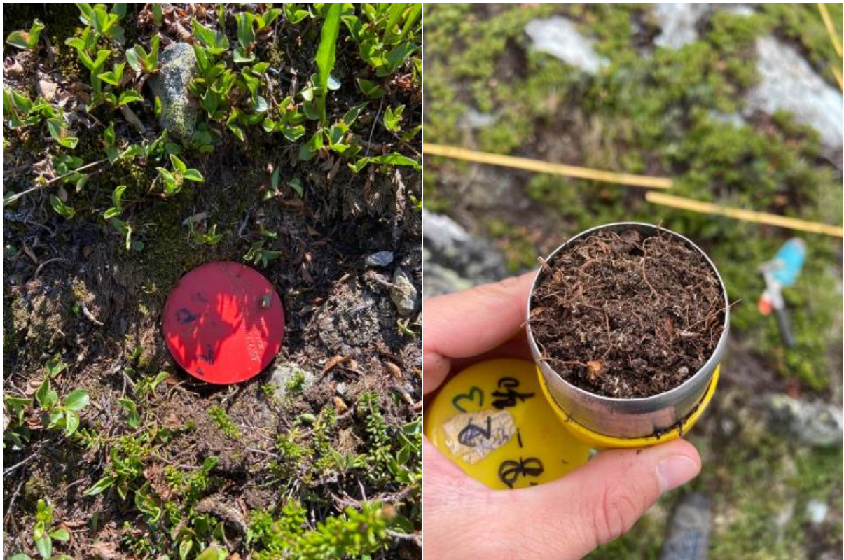
Figure 8: Example of placing a soil sample cylinder into the soil (left) and when the soil sample was taken out of the soil (right) (picture by Dick van de Lisdonk).
