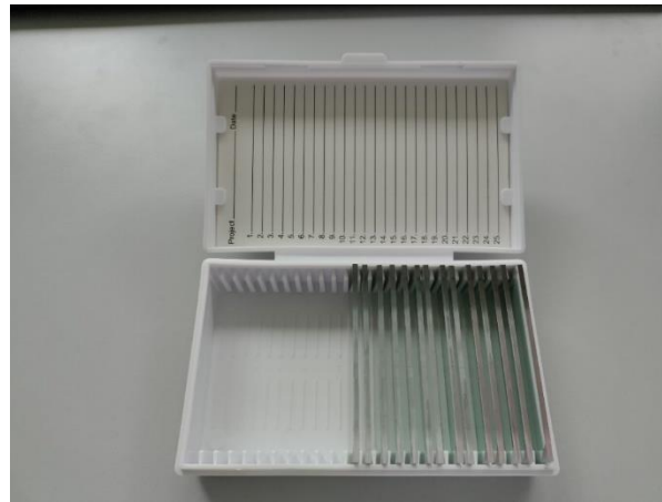
Figure 11 - Photograph of polypropylene carrier for microscopy slides
