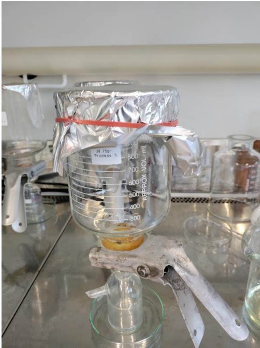
Figure 6 - Example of sealed filtration unit
